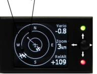
The green LED describes the GPS status of the Flarm unit: flashing means GPS status is bad. The red LED is active exclusively during warning status.
