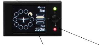
The direction of the impacting glider is marked with a **yellow big** dot on the display and the **red** LED becomes active (flashing).
