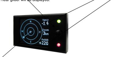
Selection is visualized with the **line** which is connecting the centre of the display and the glider symbol. If the near glider is also a member of the list of customized gliders, its ID will appear in the upper-left corner.
